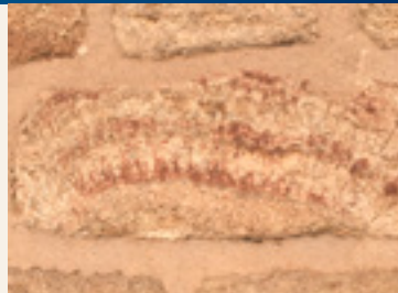
Part of a stromatolite as building stone of the
